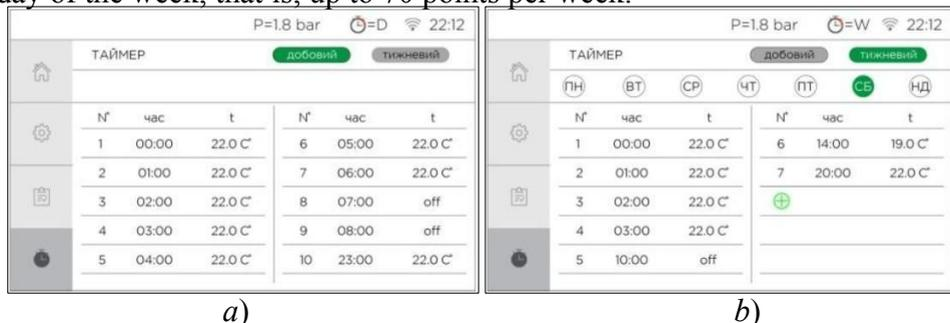
Figure 14.15 — ‘**Timer**’ submenu: a) — ‘**daily**’ type; b) — ‘**weekly**’ type
