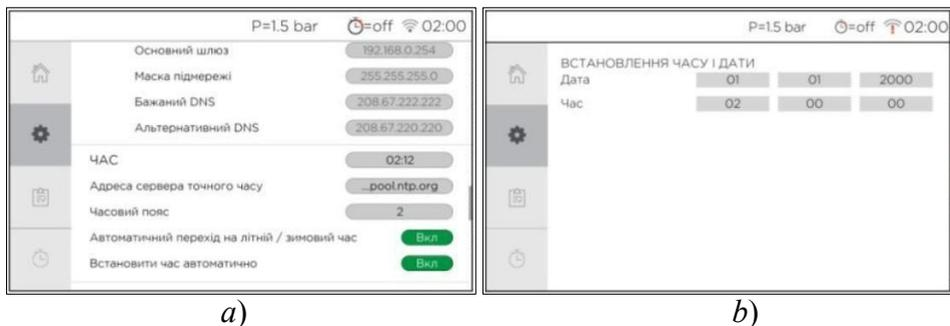
Figure 14.10 — ‘TIME’ section: *a)* — all available fields of the section; *b)* — setting the date and time
