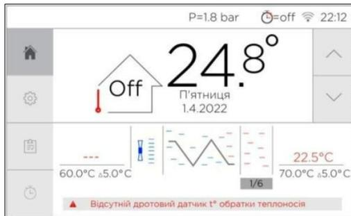
Figure 14.20 — Display of blocked and missing sensors
