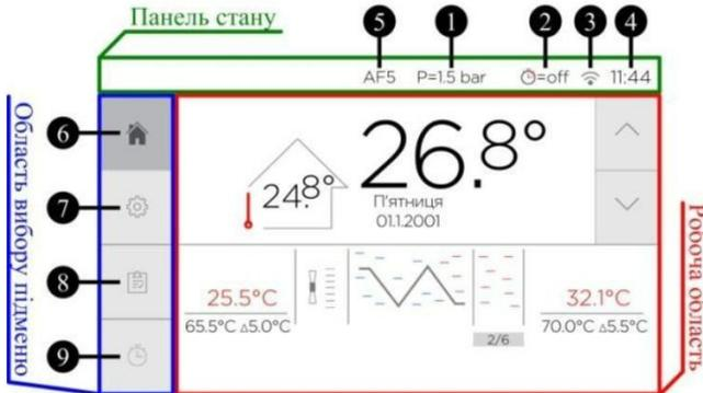
Figure 14.1 — Main areas of the boiler interface
