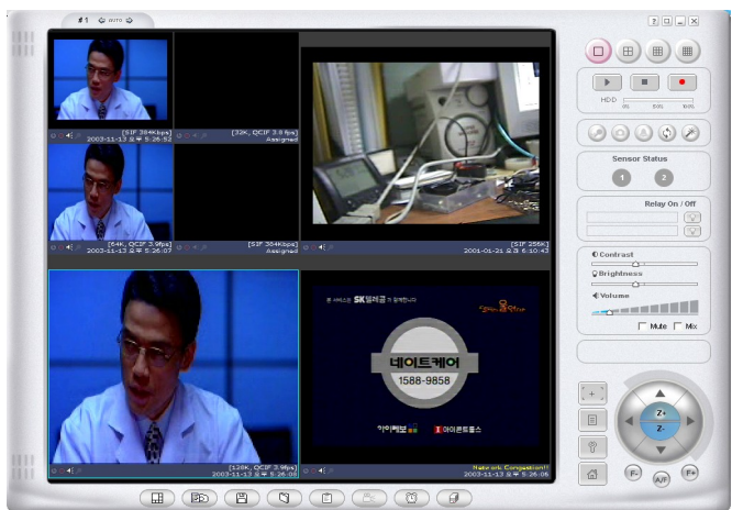
Figure 5-1. Select display channel and click "Camera Admin" button for Log on to administrative mode from "i-NVR"
