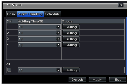
Fig 5-17 Alarm Configuration-Sensor-Alarm Handling
